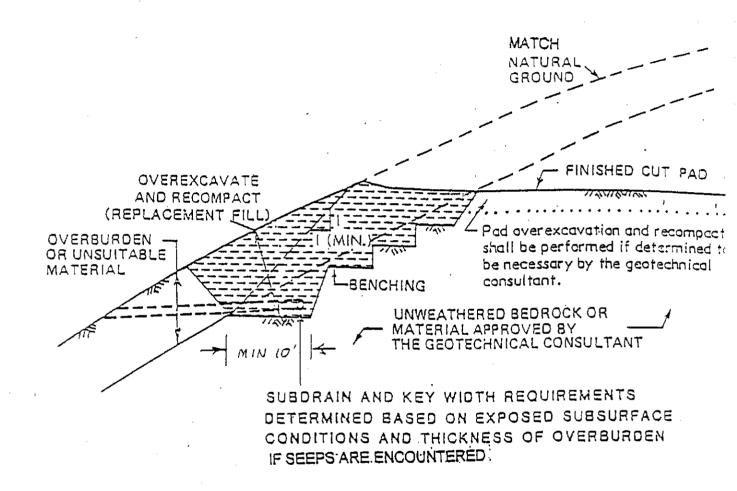
NOTE: All soil compaction should be performed to 90 percent of maximum Density as obtained by ASTM D1557-91 (5-layer) method of compaction.
