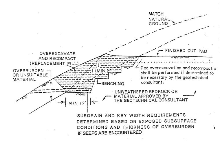
NOTE: All soil compaction should be performed to 90 percent of maximum Density as obtained by ASTM D1557-91 (5-layer) method of compaction.
