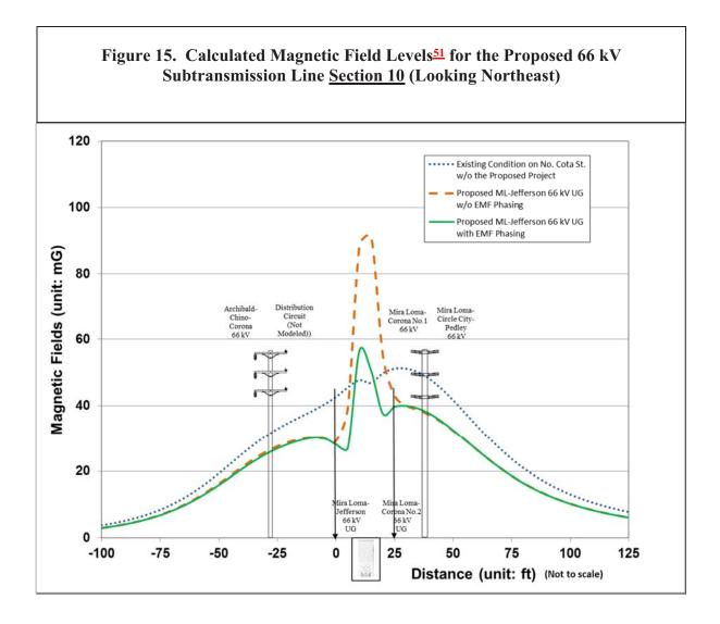
**Recommendations for** <u>Section 10</u>: The proposed design includes no-cost field reduction measures. Because the proposed design already incorporates measures meeting or exceeding SCE's preferred design criteria, no further low-cost field reduction measures are recommended.
