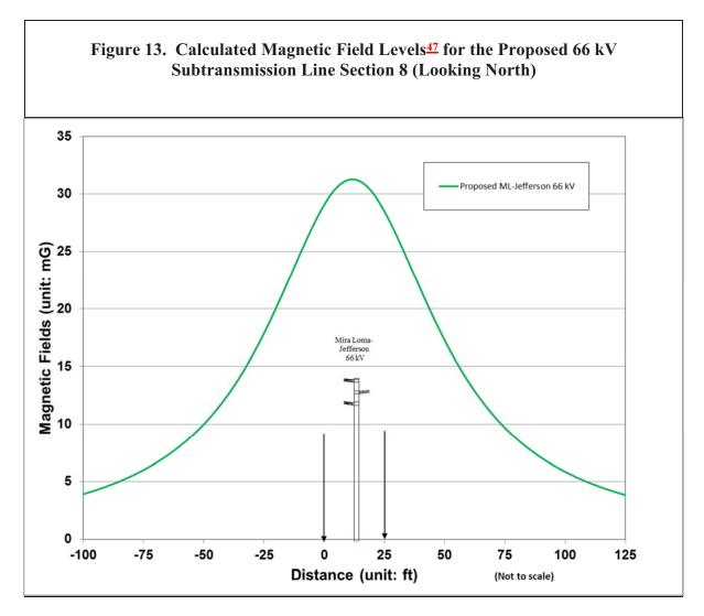
**Recommendations for** <u>Section 8</u>: The proposed design includes low-cost field reduction measure of using transposition structures to roll the phases from Section 7 recommended phasing to Section 9 recommended phasing. This measure would achieve more than 15% of magnetic field reduction at edges of the ROW in Section 9. It is recommended to adopt this low-cost magnetic field reduction measure.
