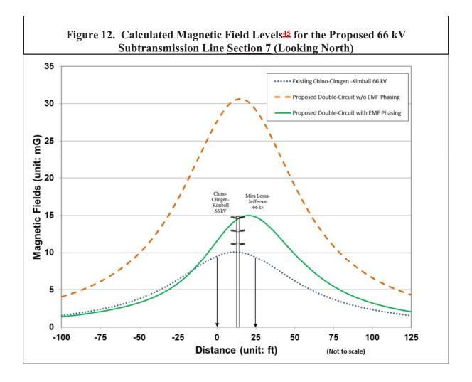
**Recommendations for** <u>Section 7</u>: The low-cost measure of re-arranging conductors for magnetic field reduction using transposition structure is recommended for this section due to nearby homes on the east side of the proposed line.
