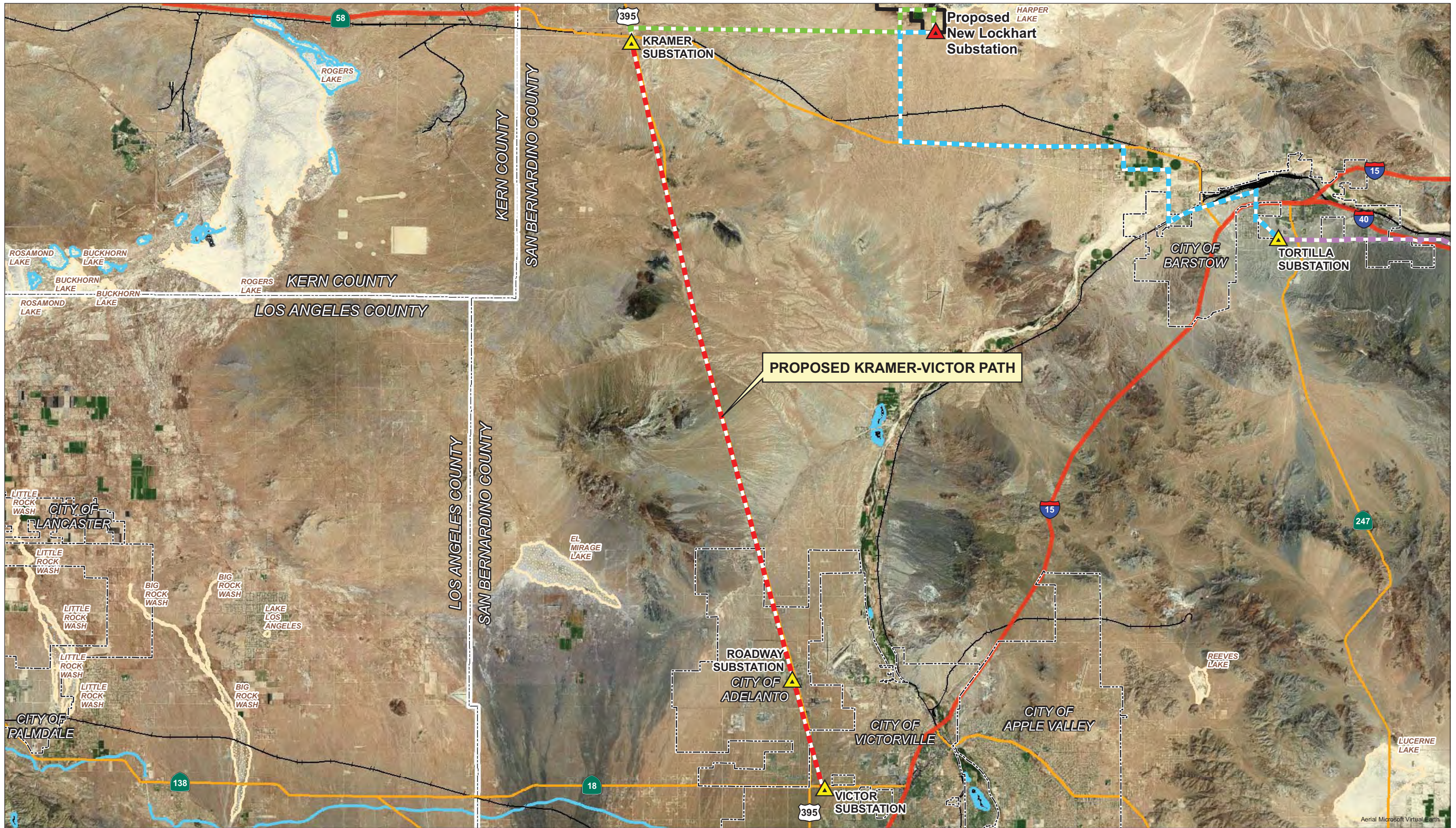
FIGURE 3-6 PROPOSED NEW TELECOMMUNICATION FIBER OPTIC CABLE CONNECTING KRAMER SUBSTATION TO VICTOR SUBSTATION
