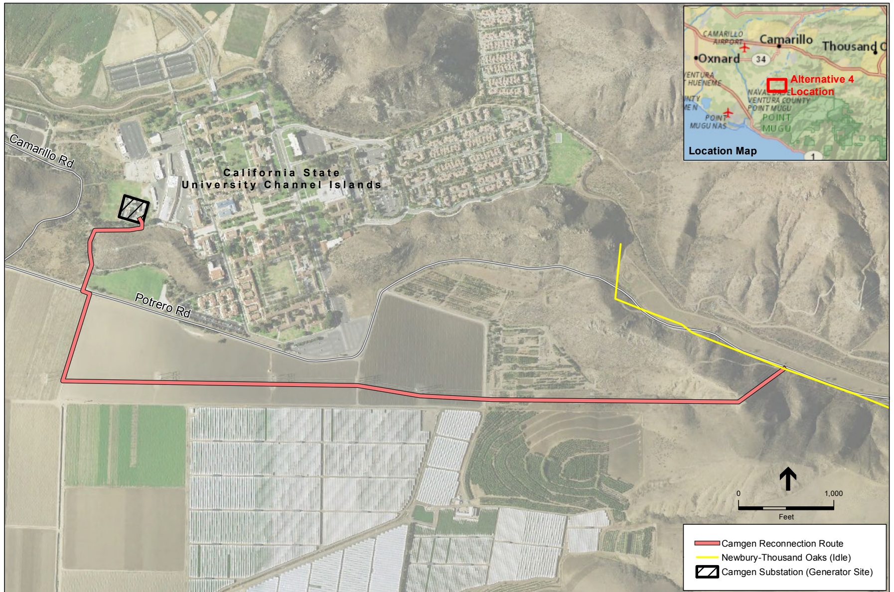
Figure 4-5 Alternative 4, Reconnect the Camgen Generator to the Moorpark System
