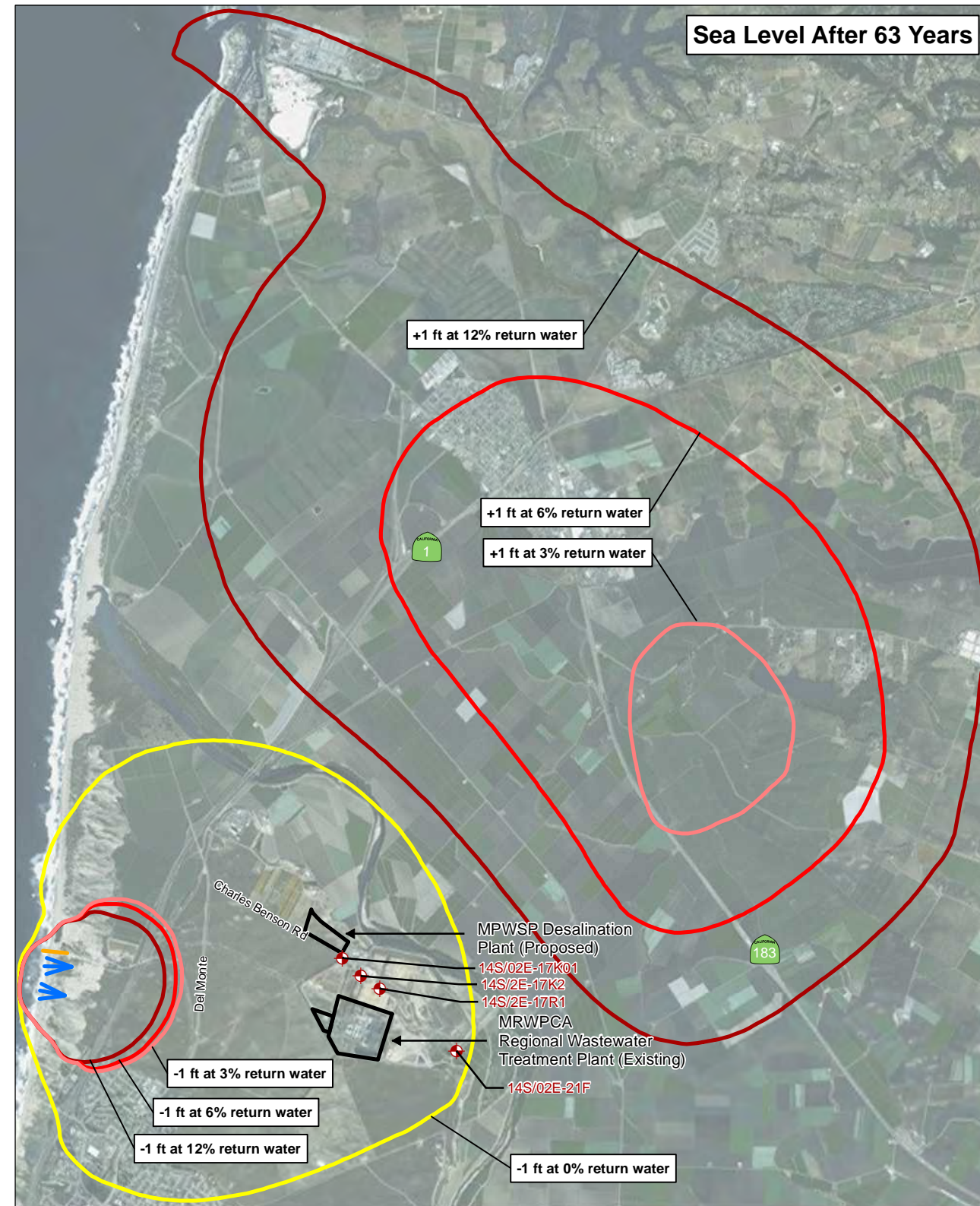
205335.01 Monterey Peninsula Water Supply Project Figure 5.5-6 Alternative 5a Site: 1-Foot Response in 180-Foot Aquifer under 15.5 MGD Pumping
