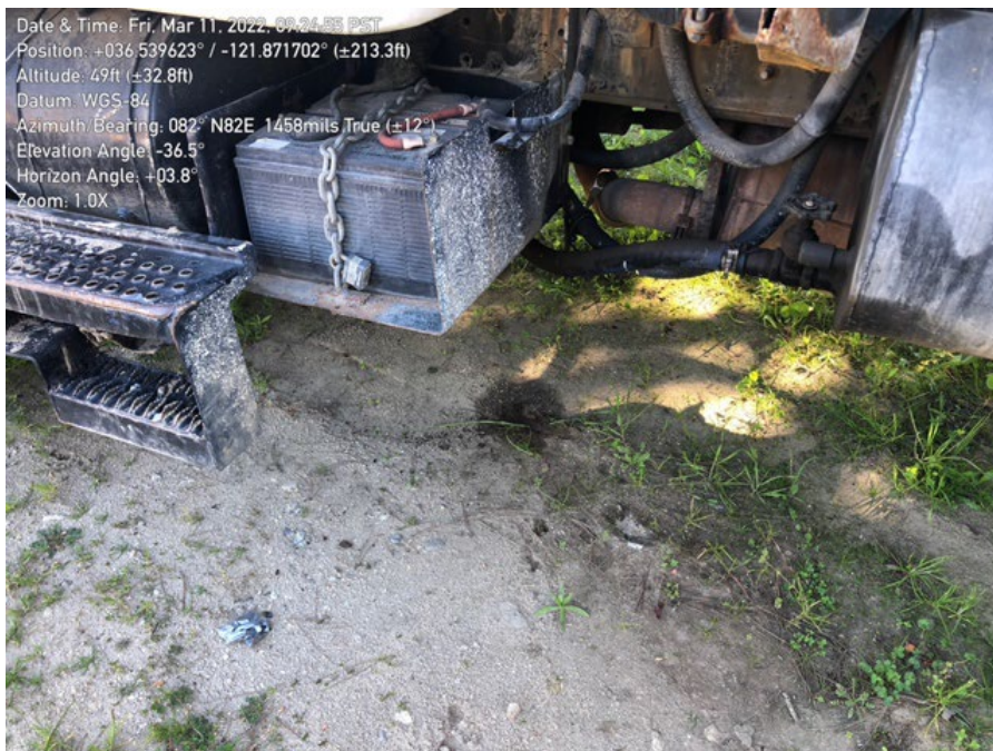
Photo 2. Minor hydraulic leak under water truck.
