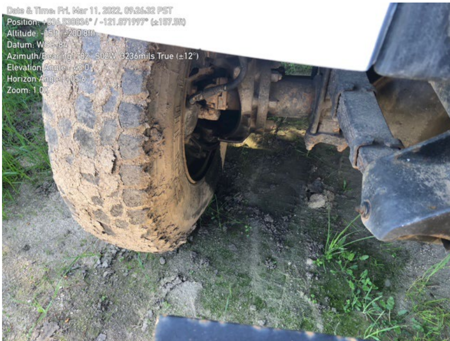
Photo 3. Minor hydraulic leak under water truck.
