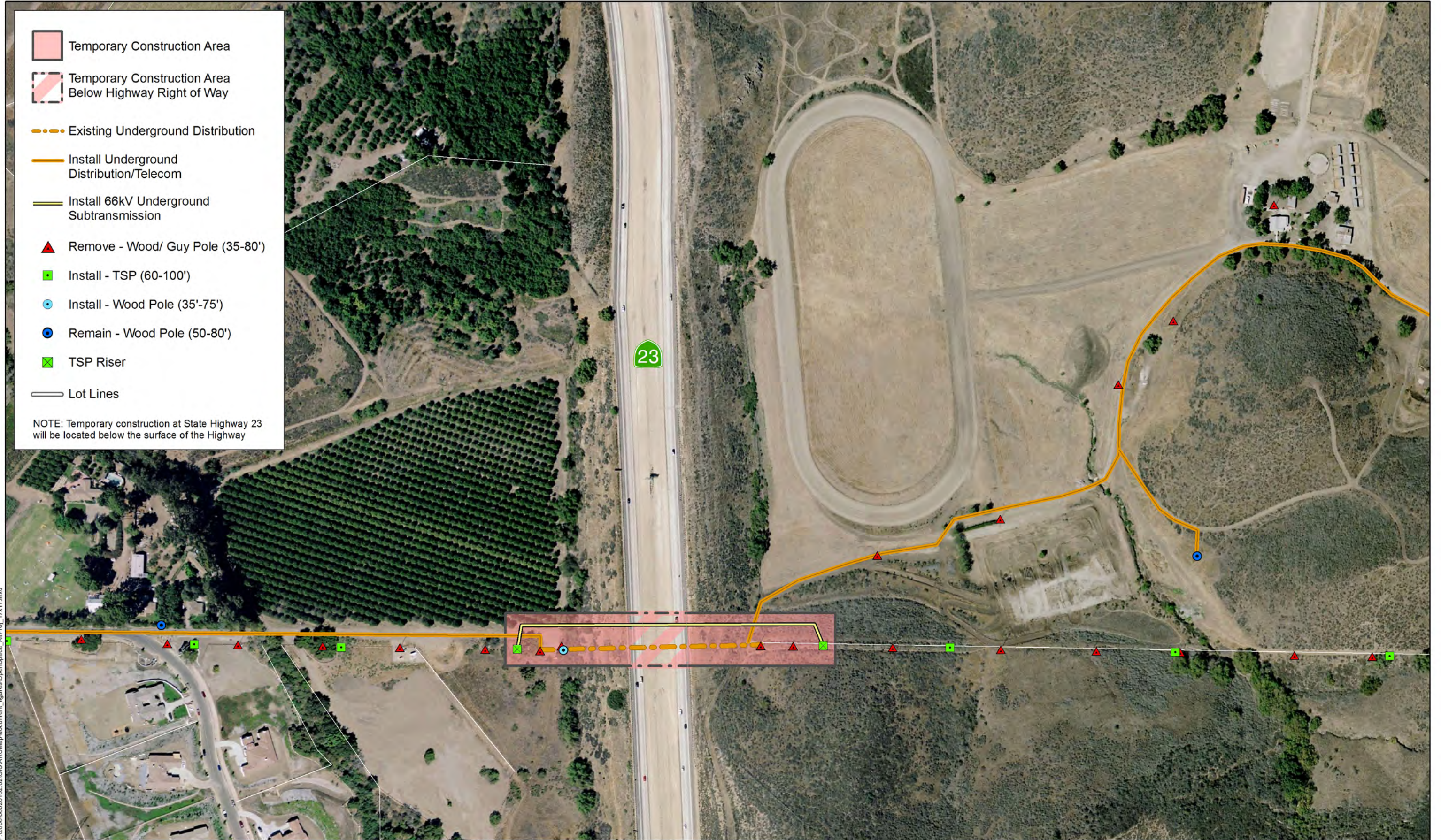
FIGURE XX: PROPOSED CONSTRUCTION AREA DUE TO UNDERGROUNDING OF 66 KV SUBTRANSMISSION LINE AT STATE HIGHWAY 23
