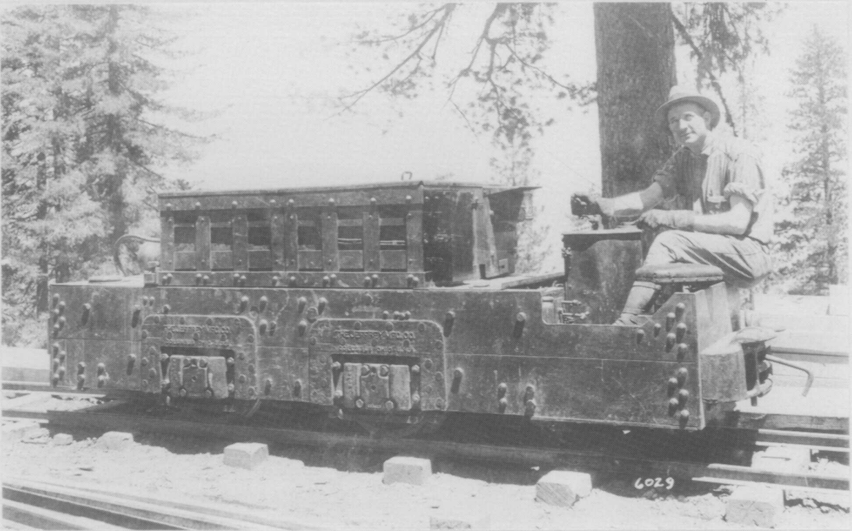
Plate 26 Storage battery locomotive, date unknown (SCE var. [a]:Album 3, No. 6029).
