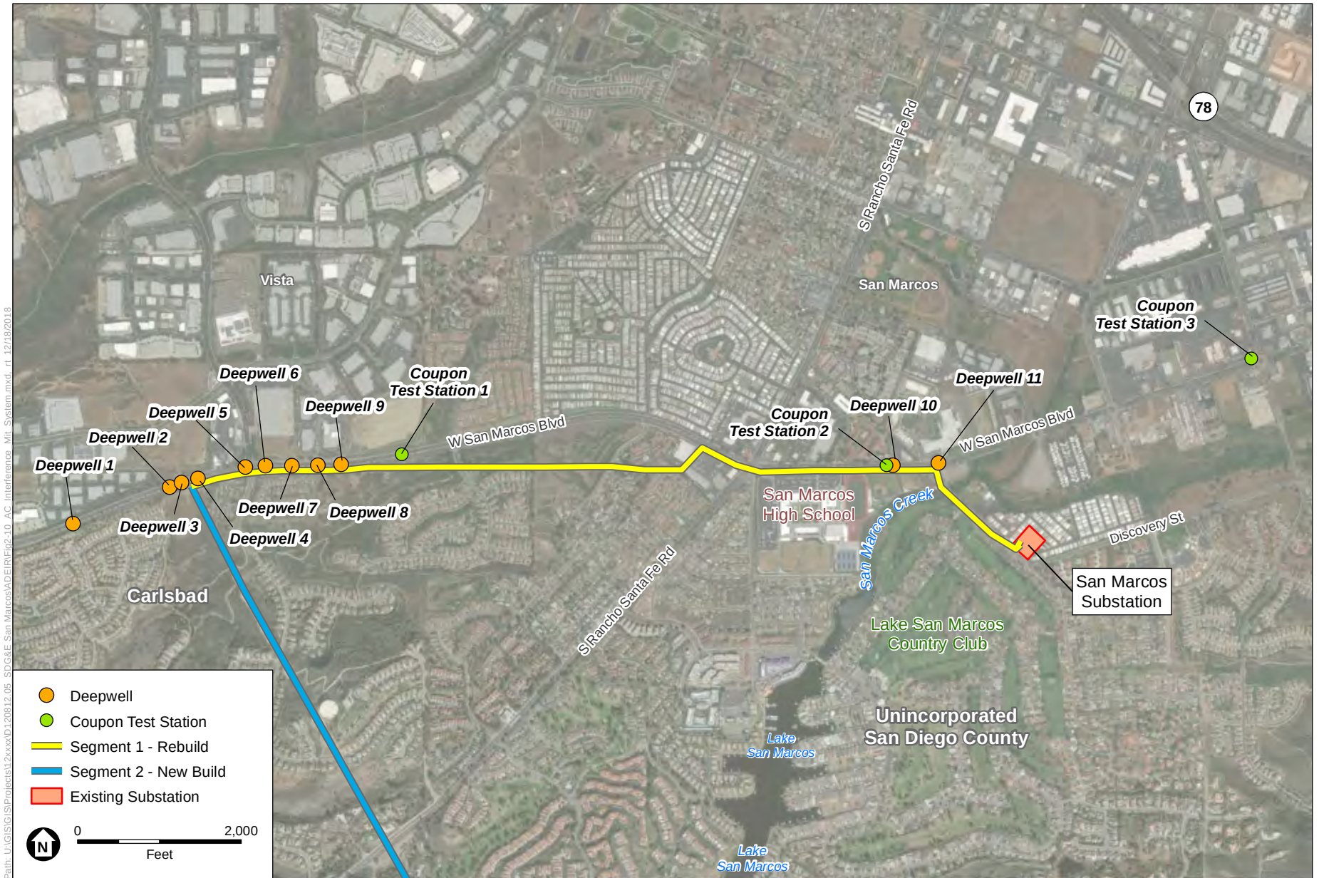
Figure 2-10 AC Interference Mitigation System
