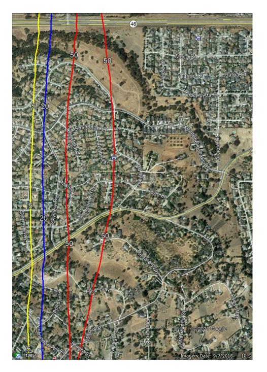
Figure 4-4 Results of Acute DPM Modeling in Micrograms per Cubic Meter Scenario 1
