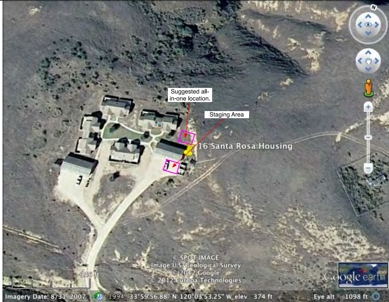
Figure 16.3: Santa Rosa Island Housing staging area. No digging required for wiring on either option. All options require no wire suspension, aboveground conduit, or trenching to connect equipment because the telecom enclosure, CITC VSAT, antenna, and solar panels would all be seated on the all-in-one solution or structure. All wiring would be affixed to the structure using cable mounts. Suggested all-in-one solution location shown.
