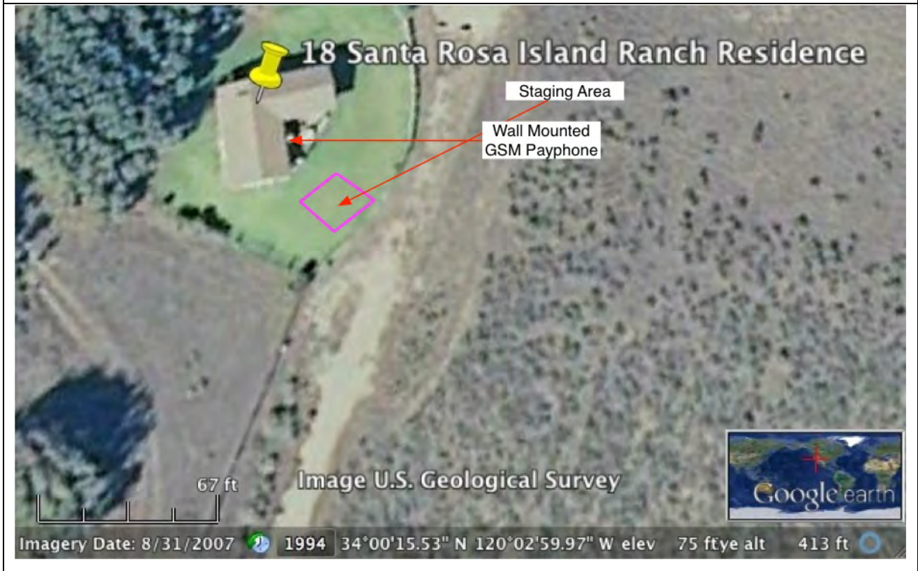
Figure 18.1: Ranch Residence staging area. No digging required for wiring. All options require no wire suspension, aboveground conduit, or trenching to connect equipment because the telecom enclosure, CITC VSAT, antenna, and solar panels are all seated on or around the structure. All wiring would be affixed to the structure using cable mounts.
