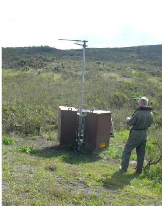
Figure 9 – A typical weather station/auxiliary outdoor equipment cabinet powered by Solar on San Miguel Island
