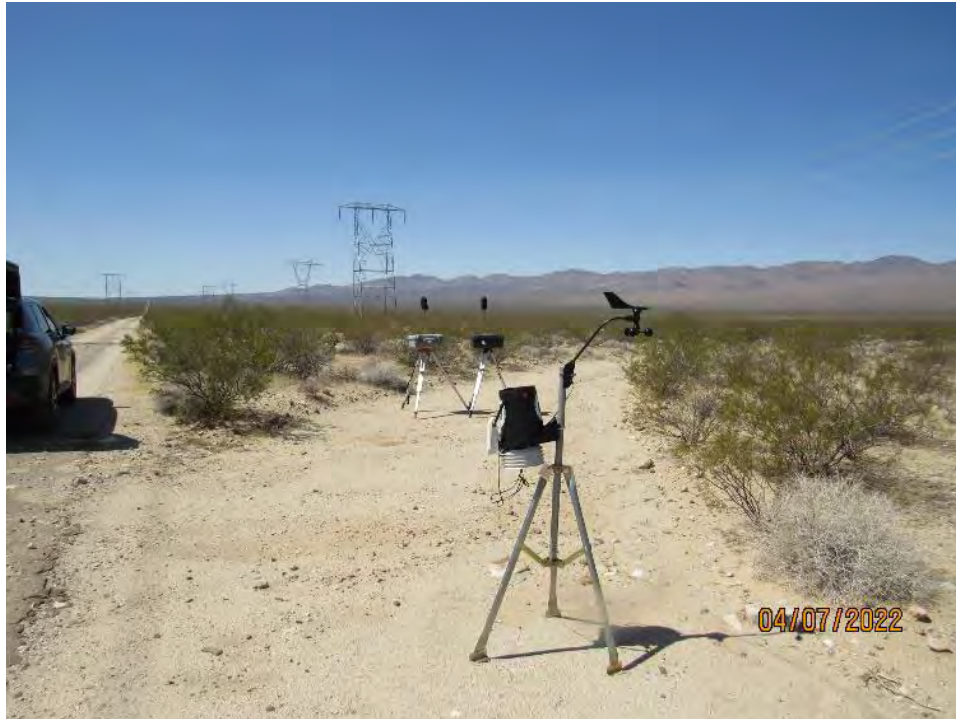
Photograph 9 - Monitors were repositioned to collect measurements at zero, fifty and one hundred meters from transmission lines in the Mojave National Preserve near Ivanpah Road and Power Line Road. Power Line Road is seen on the left side of this image.
