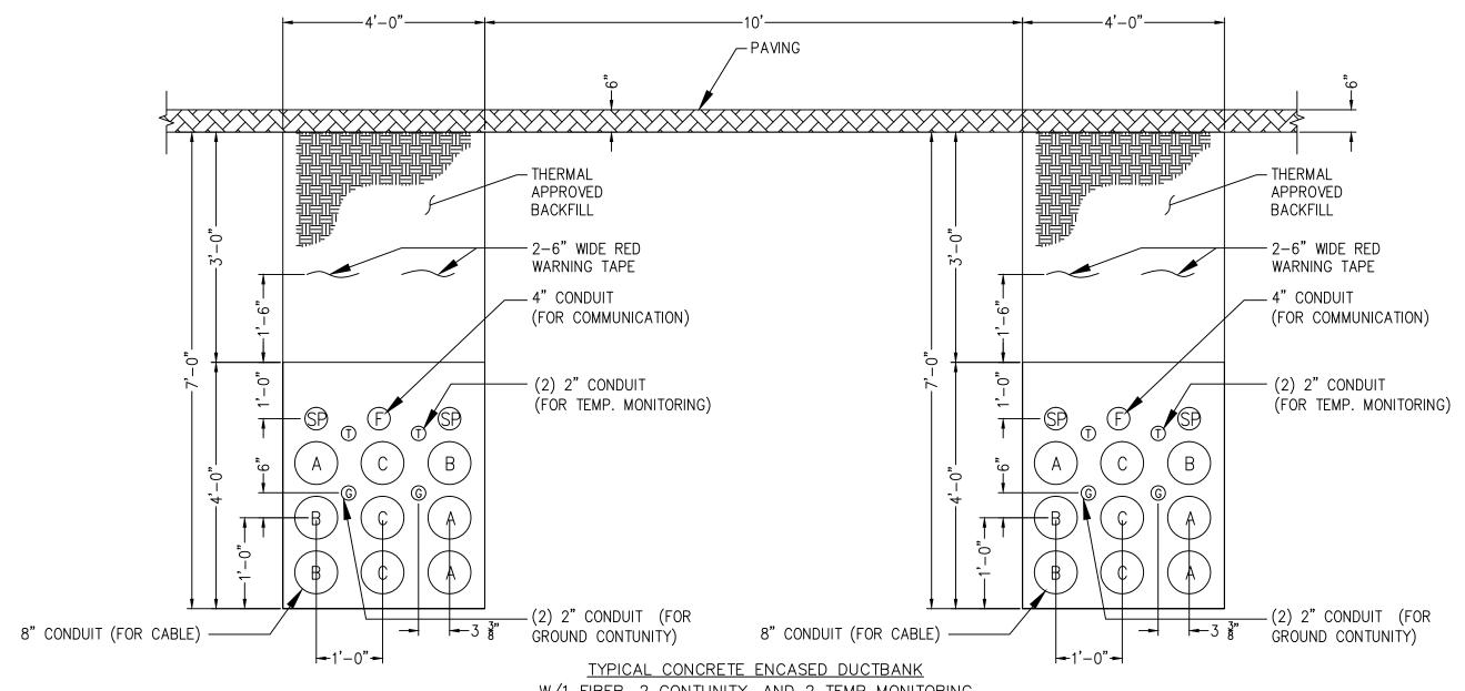
W/1 FIBER, 2 CONTUNITY, AND 2 TEMP MONITORING CONDUITS FACING UP STATION NOT TO SCALE
