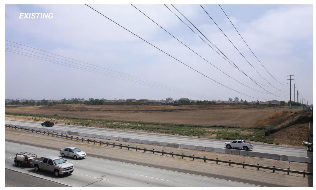
Existing transmission line along 68th St includes six (6) high voltage conductors and four (4) distribution voltage conductors.
