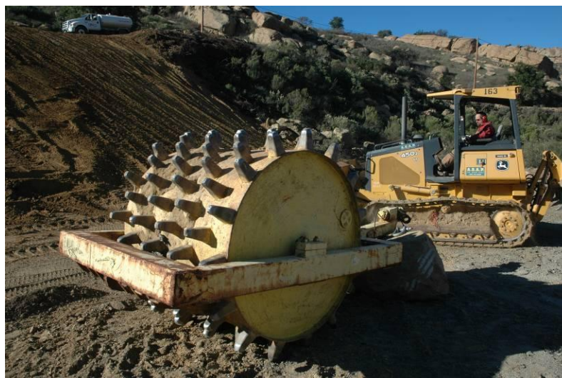
Sheepsfoot used for soil preparation
