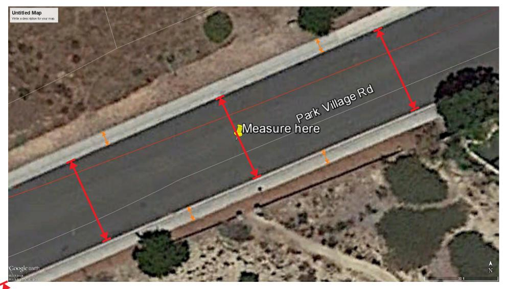
Road measurements to be accomplished with a Spectra Precision Laser (+/- 1/8"). Tape measure will be used if the crown of the road blocks line-of-sight. Measurement will be from vertical portion of curb on each side of the road and will include the approximate 1' concrete gutter (see page 2).
