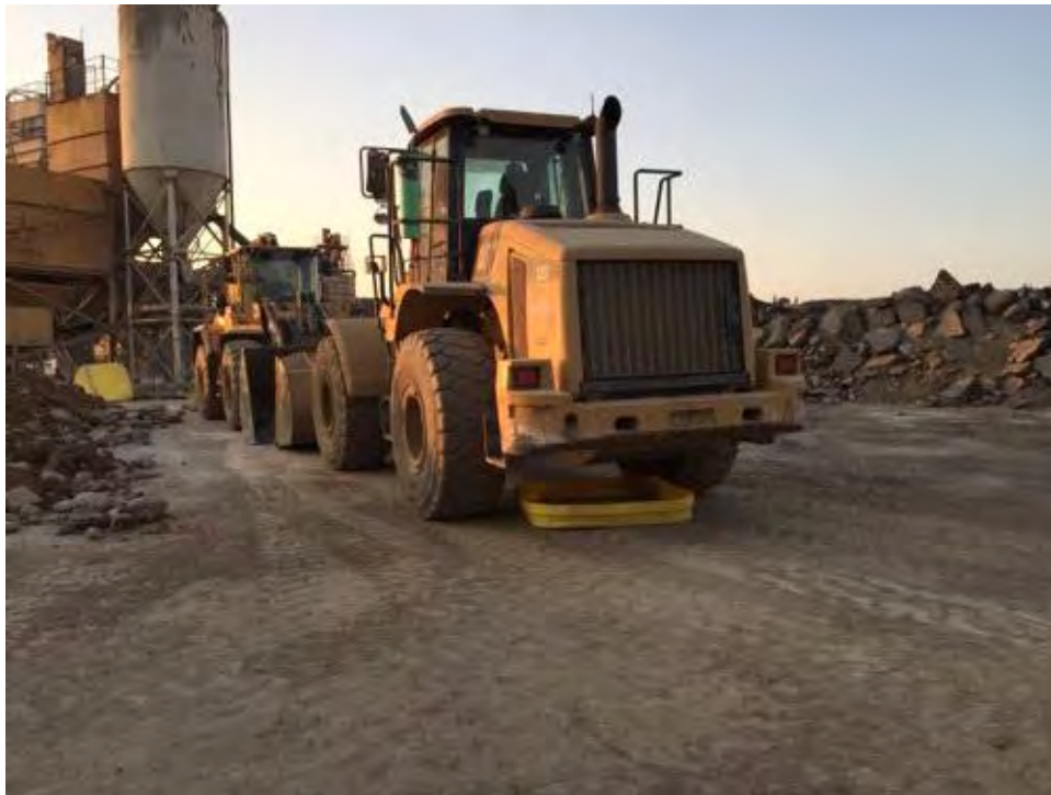
Caption Drip pans in place under equipment at construction yard off of Camino Ruiz.
