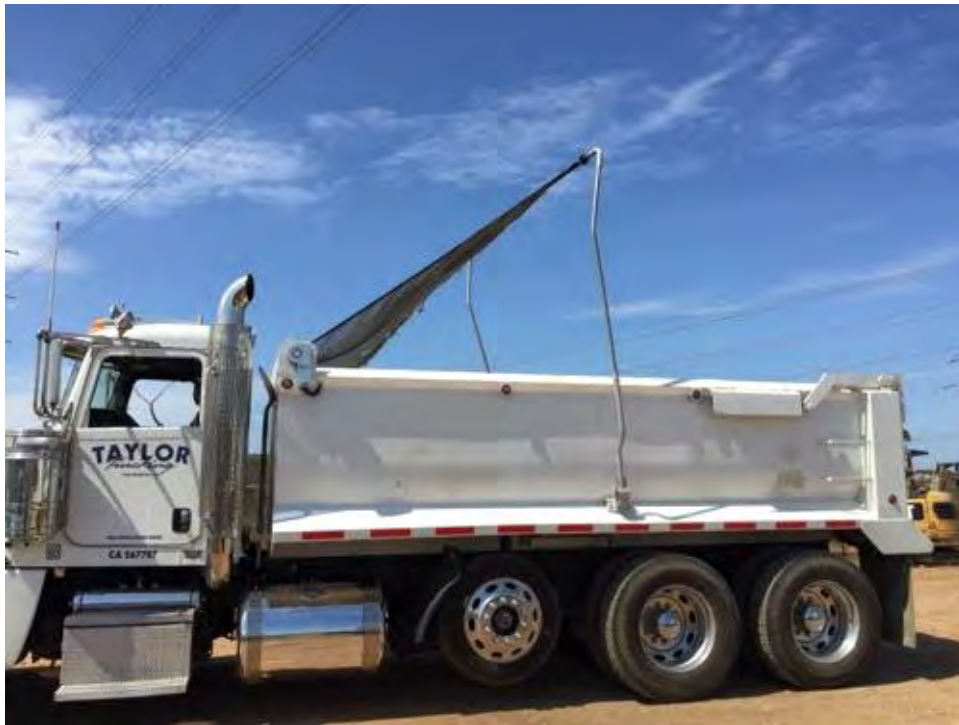
Caption Dump truck covering the fill before exiting Pole 03 site .
