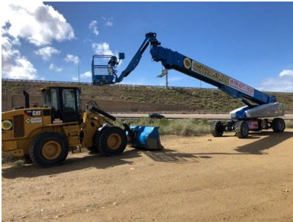
Caption No drip pan on either piece of equipment.
