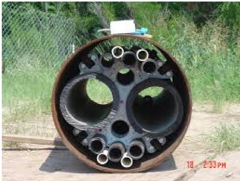
Figure 4 – Typical Jack and Bore Installation
