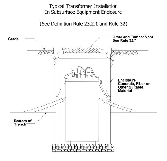
Figure 18 Typical Transformer Installation in Subsurface Equipment Location (See Definition Rule 23.4 and Rule 32)
