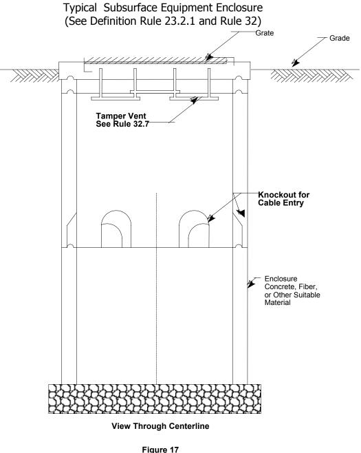
Figure 17 Typical Subsurface Equipment Enclosure (See Definition Rule 23.4 and Rule 32) 4. Figure 18 is added to appendix B of the General Order to appear as follows:
